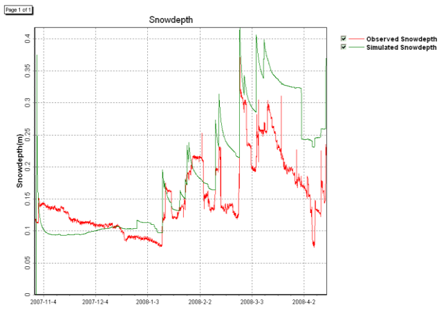
Fig. 5. The observed and simulated snow depth of the Binggou watershed from date to date with sublimation process included.
